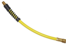
33204 91486357 Hose whip, 3/8" NPT, 10 mm inside diameter, 30 cm (1 ft)
